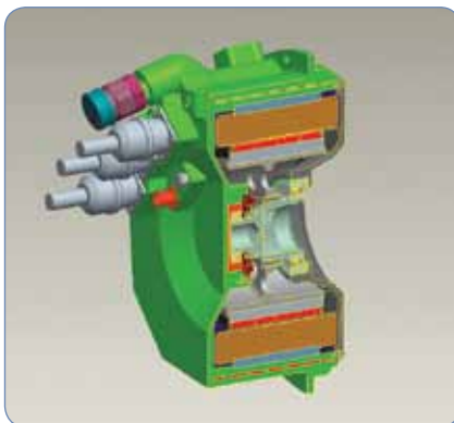
200 kW electric starter/generator
